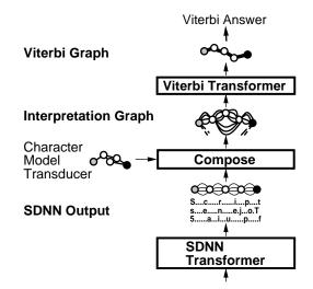
Fig. 24. A Graph Transformer pulls out the best interpretation from the output of the SDNN.
