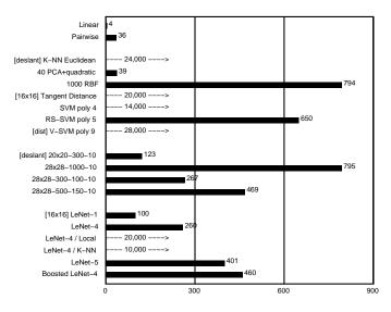
Fig. 11. Number of multiply-accumulate operations for the recognition of a single character starting with a size-normalized image.
