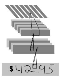
Fig. 23. A Space Displacement Neural Network is a convolutional network that has been replicated over a wide input field.
