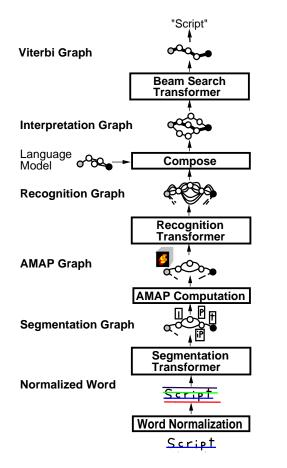
Fig. 30. An on-line handwriting recognition GTN based on heuristic over-segmentation  $\$
