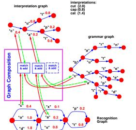
Fig. 28. Example of composition of the recognition graph with the grammar graph in order to build an interpretation that is consistent with both of them. During the forward propagation (dark arrows), the methods **check** and **fprop** are used. Gradients (dashed arrows) are back-propagated with the application of the method **bprop**.
