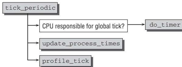
Figure 15-11: Code flow diagram for tick_periodic .
