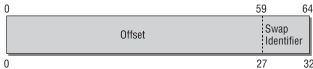
Figure 18-6: Components of an architecture-independent swap identifier.
