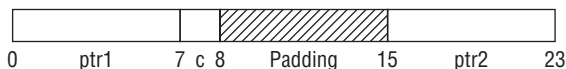
Figure C-4: The compiler automatically inserts padding space into structures to make them fulfill alignment requirements.
