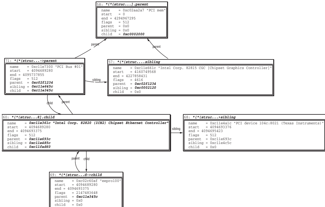
Figure 6-21: Allocated resources of a PCI network card.
