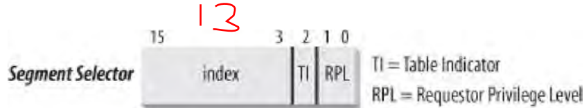
Figure 2-2. Segment Selector format
