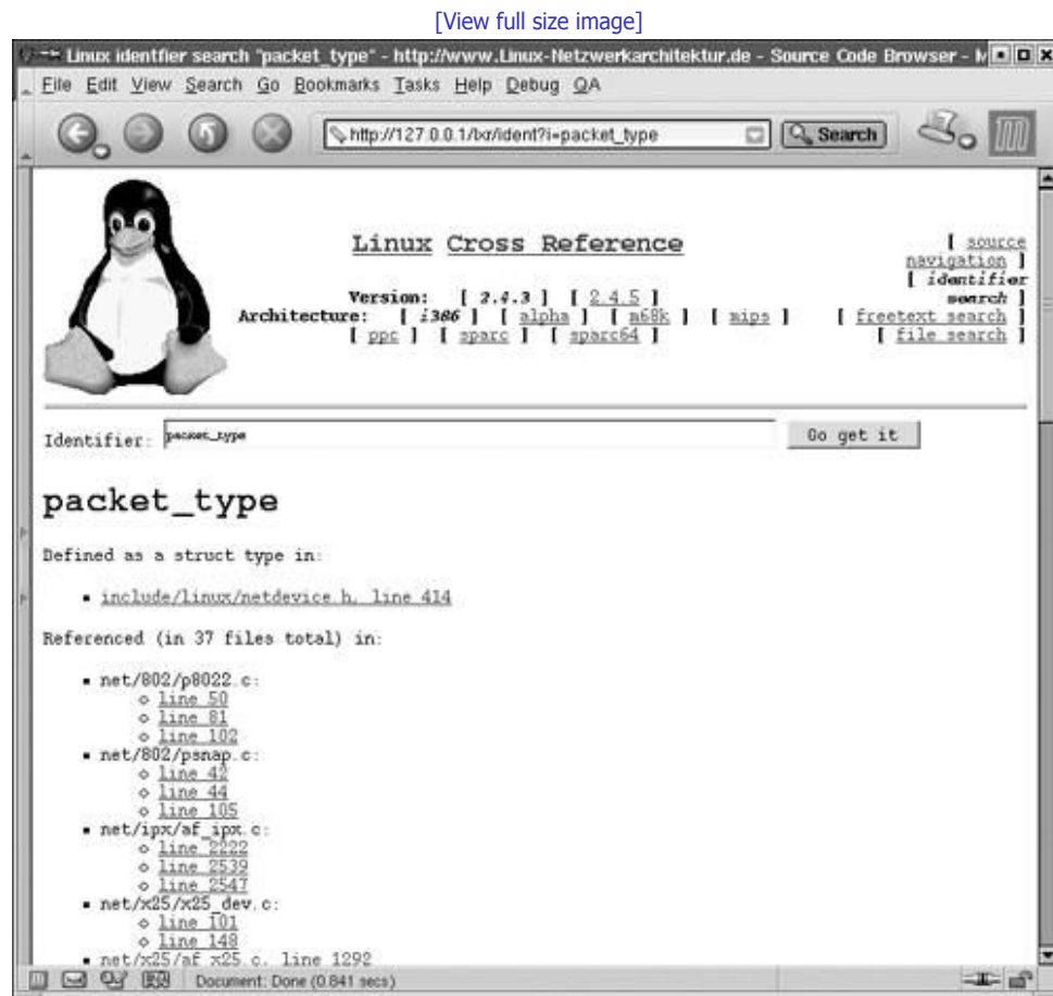
Figure A-4. Information stored for the C structure packet_type
