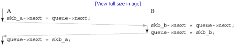
Figure 2-3. (Undesired) result of the unprotected operations of activities A and B.
