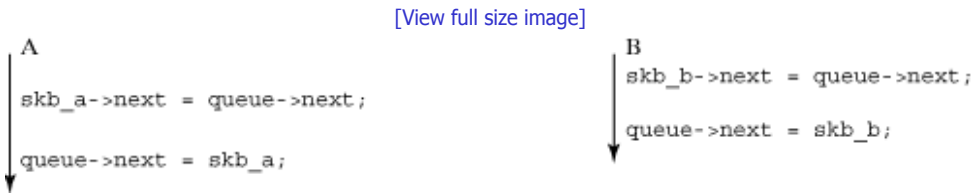
Figure 2-4. Parallel operations of the activities A and B in the critical section.
