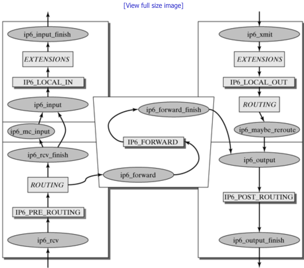
Figure 23-3. IPv6 implementation in the Linux kernel.
