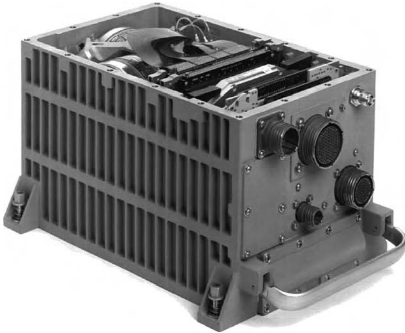
FIGURE 12.4 GPS-inertial navigator. The inertial instruments are mounted at the rear with two laser gyroscopes and electrical connectors visible. The input-output board is next from the rear; it includes MIL-STD-1553 and RS-422 buses. The computer board is next closest to the observer, and the power supply is in front. Between is the single-board shielded GPS receiver. Round connectors on the front are for signals and electric power. A battery is in the case behind the handle. Weight 10 kg, power consumption 40 watts. This navigation set is used in many military aircraft and, without the GPS receiver, in Airbus airliners. (Photo courtesy of Northrop-Grumman Corporation.)
