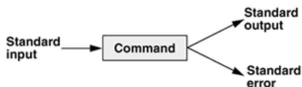
Figure 5-3. The command does not know where standard input comes from or where standard output and standard error go
