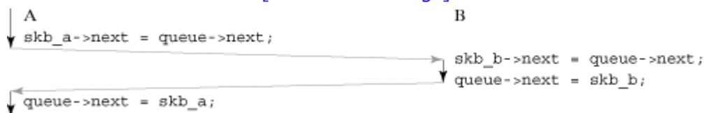
Figure 2-3. (Undesired) result of the unprotected operations of activities A and B.
