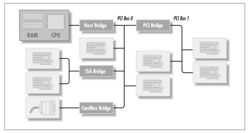
Figure 15-1. Layout of a Typical PCI System
