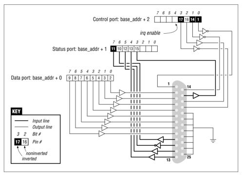
Figure 8-1. The pinout of the parallel port
