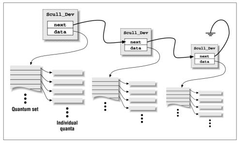
Figure 3-1. The layout of a scull device
