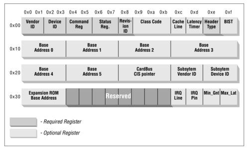
Figure 15-2. The standardized PCI configuration registers
