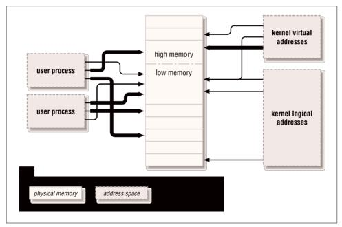
Figure 13-1. Address types used in Linux
