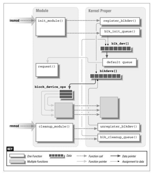
Figure 12-1. Registering a Block Device Driver
