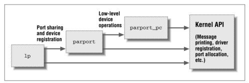
Figure 2-2. Stacking of parallel port driver modules
