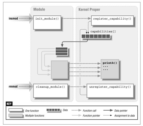
Figure 2-1. Linking a module to the kernel
