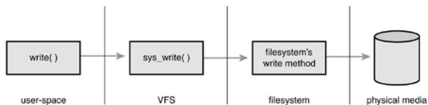
Figure 12.2. The flow of data from user-space issuing a write() call, through the VFS's generic system call, into the filesystem's specific write method, and finally arriving at the physical media.
