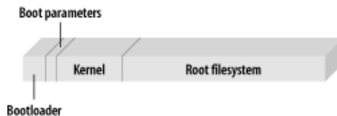
Figure 2-5. Typical solid state storage device layout
