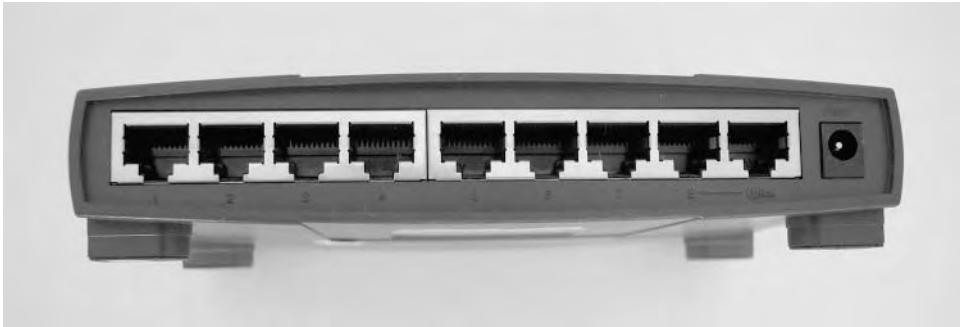
Figure 2-4: A hub has multiple ports for connecting interfaces to a network.
