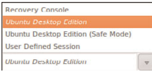
FIGURE 3.5 Use the Select Session option to select the desktop environment of your choice before you log in.
