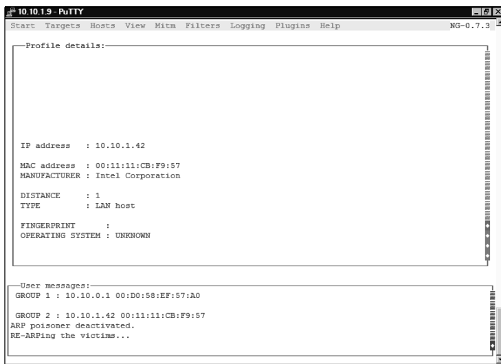
Figure 6.8 Ettercap Successfully Restoring the Mangled ARP Tables
