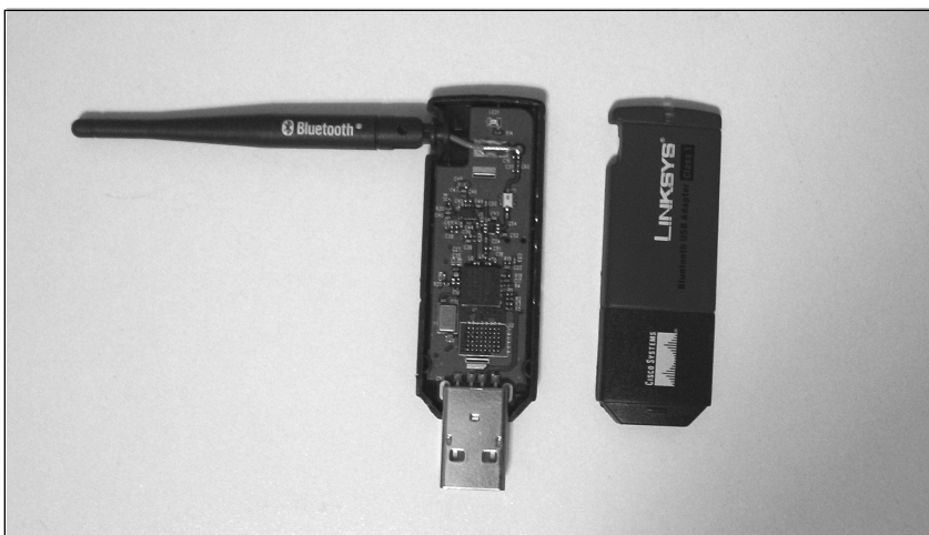
Figure 2.10 Opening the Bluetooth Adapter Case
