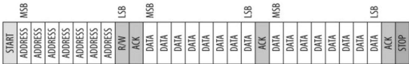
Figure 13-2. Format of a transaction on an I 2 C bus
