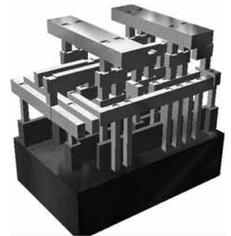
FIGURE 6.3 Graphical representation of the layers of an IC.
