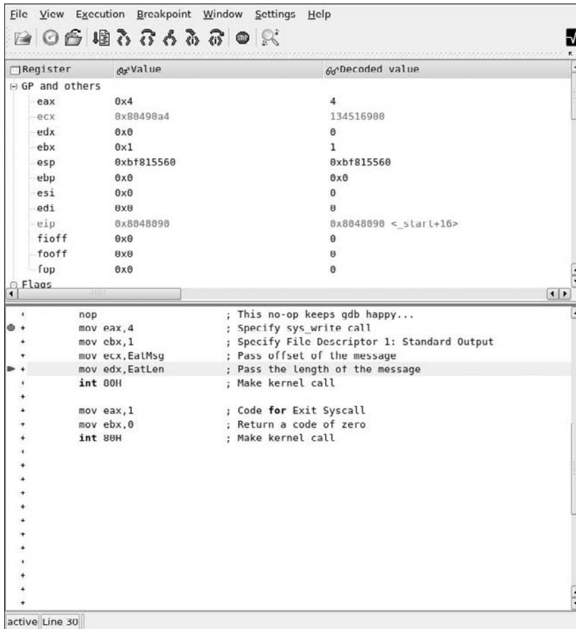
Figure 5-15: Moving a memory address into a register
