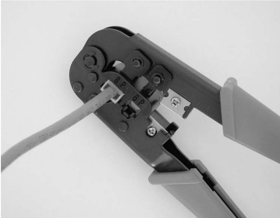
Figure 2-9: A crimping tool attaches the connector to the cable.
