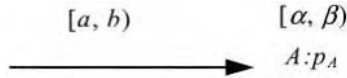
Fig. 4. A job annotated with its possible execution, start time and current priority.
