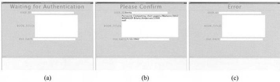
Fig. 6. Screen dump of authentication results: (a) waiting for authentication; (b) authentication is successfully done; (c) authentication failure occurs
