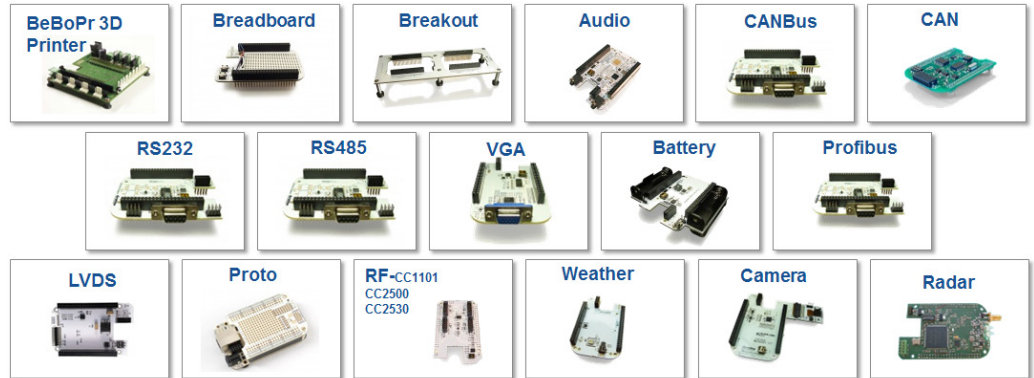
Figure 3. Cape plug-in boards easily expand the capabilities of BeagleBone Black.
