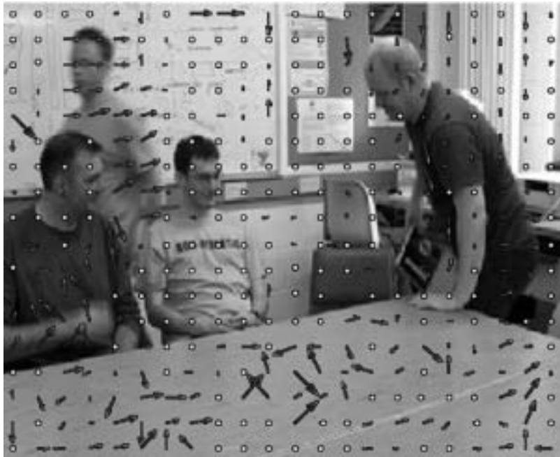
Figure 3.55 16 \times 16 motion vectors (superimposed on frame)
