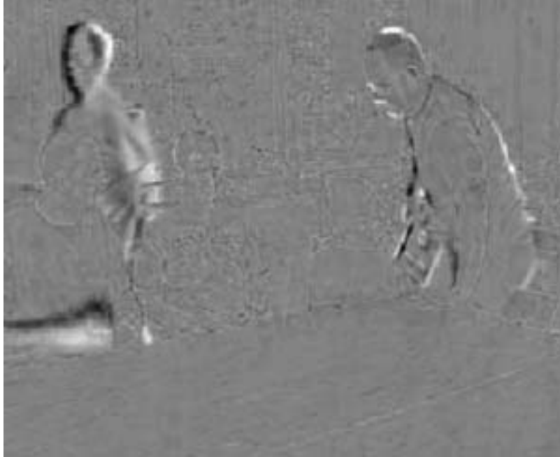
Figure 3.54 Residual F_n - F'_{n-1} (no motion compensation)
