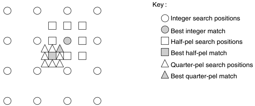
Figure 3.18 Integer, half-pixel and quarter-pixel motion estimation
