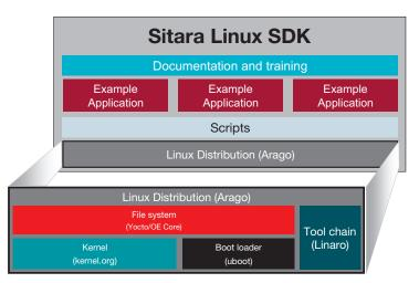
Figure 2: TI's Sitara™ Linux™ SDK and Arago Linux distribution
